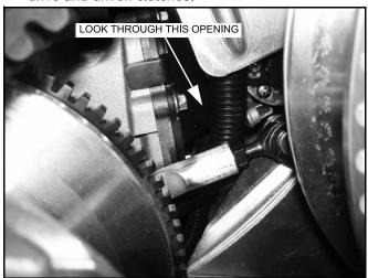
Using a mirror and a flash light, visually inspect the current oil pump setting. The scribe mark should be aligned with the point of the lever notch when the throttle plates are closed.
