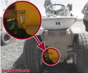
Serial number plate mounted on the rear drive housing.
