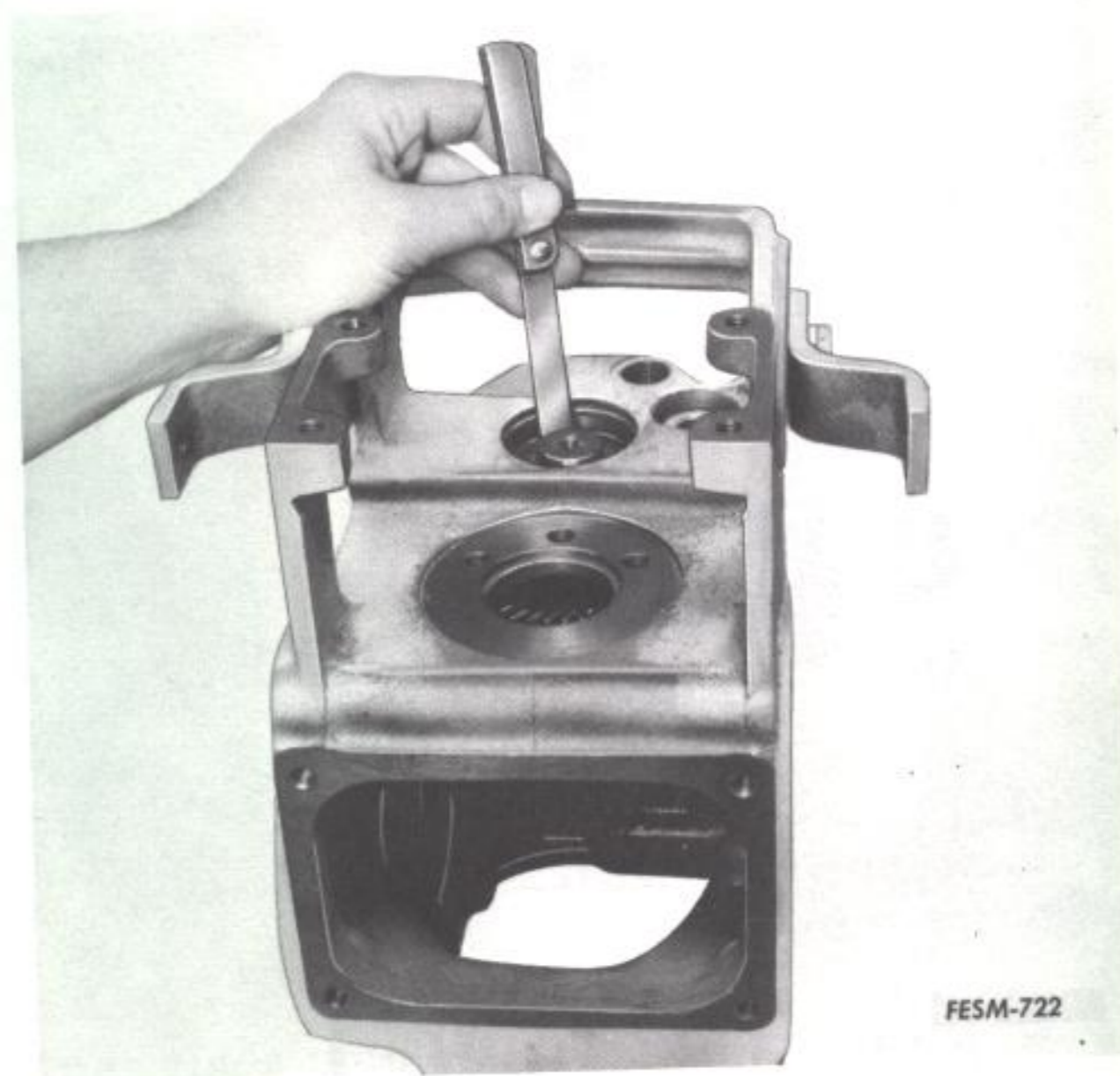
Illustr. 2-72. Measuring snap ring groove gap.
