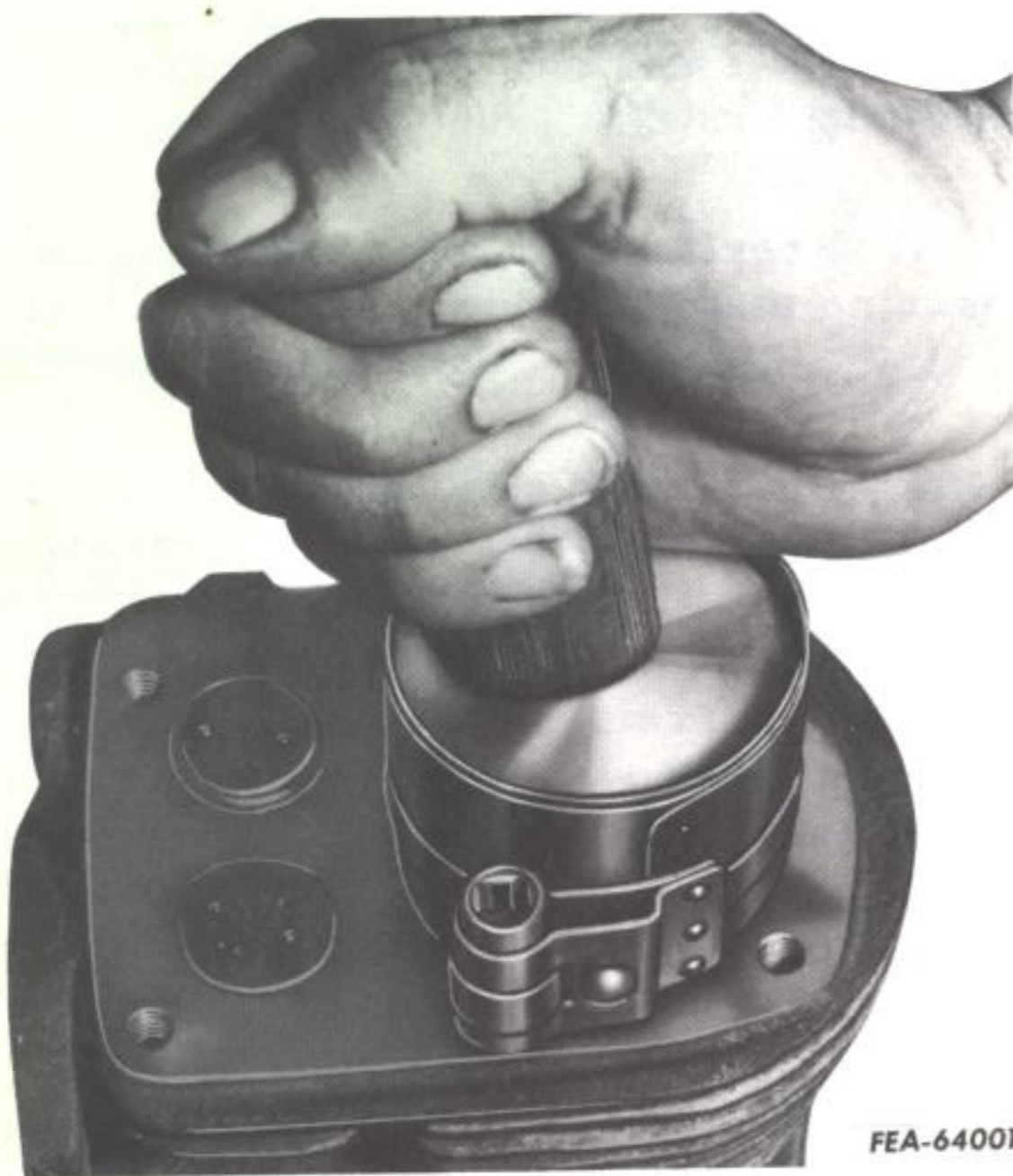
Illust. 1-17. Installing piston assembly.
