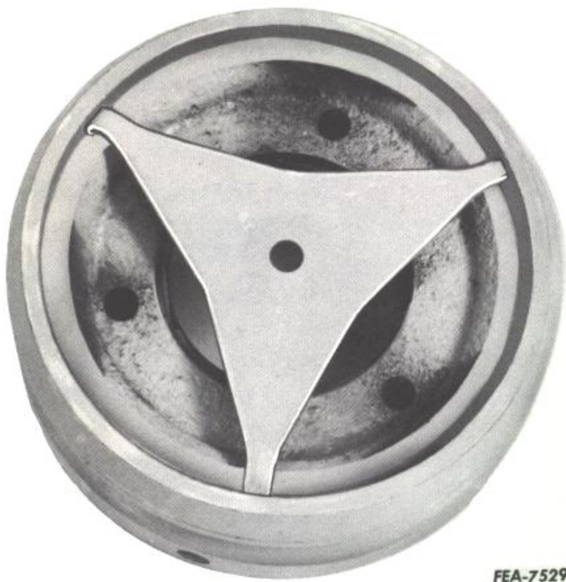
Illust. 2-84. Pressure spring located on pulley.
