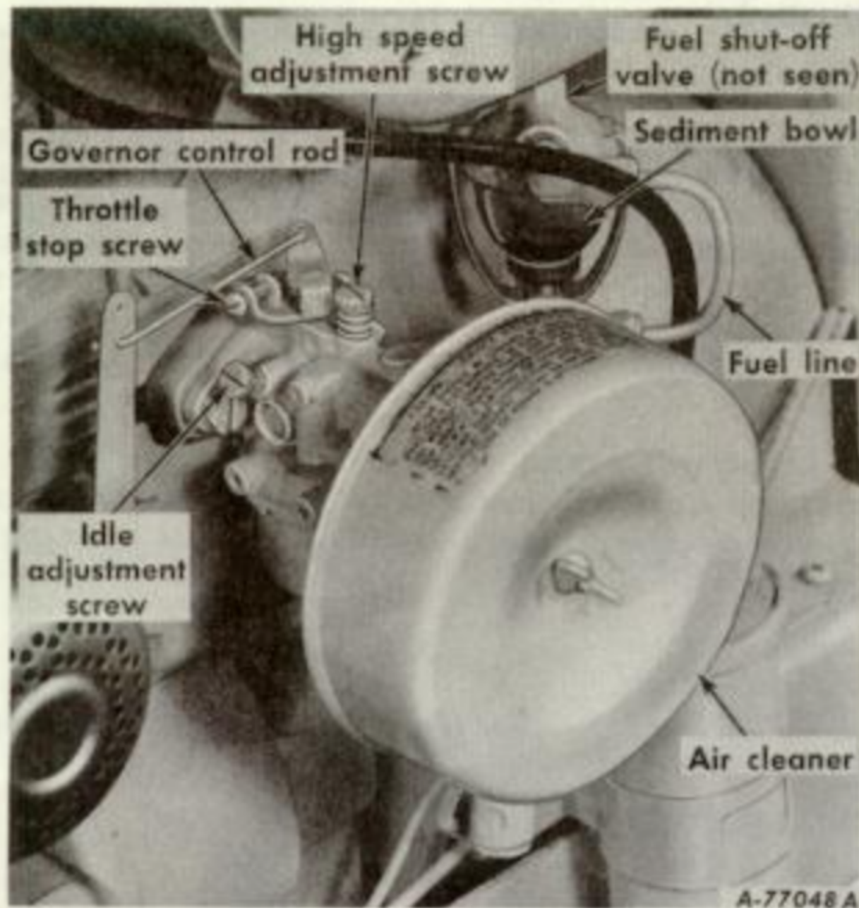
Illust. 9 Carburetor and fuel strainer. (International Cub Cadet 72 Tractor)
