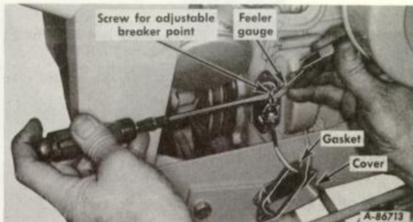
Illust. 17A Adjusting the breaker points. Set gap at .020-inch.
