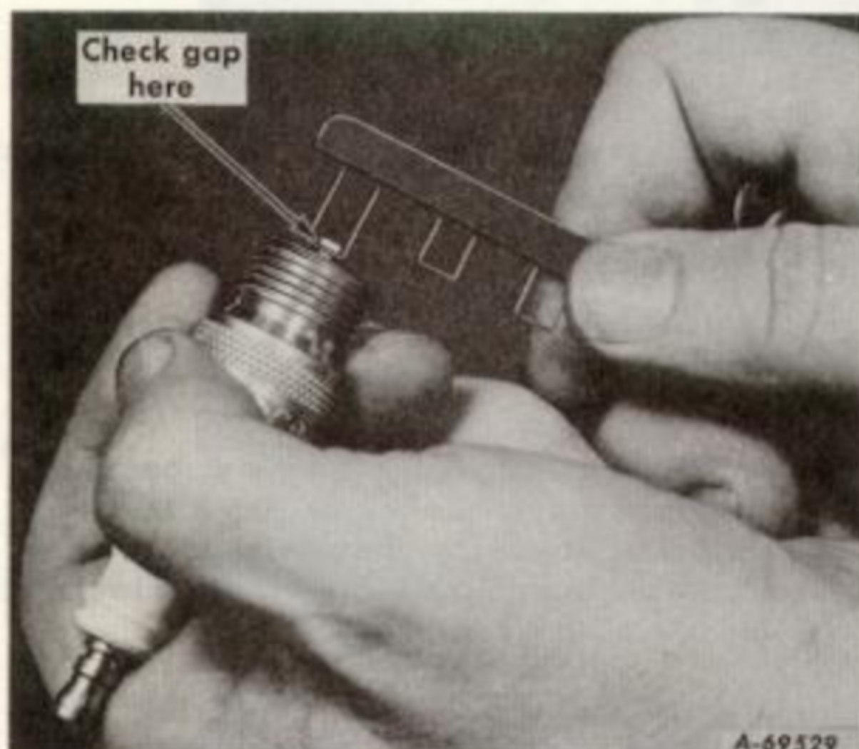
Illust. 17 Checking the spark plug gap. Set gap at .025-inch.
